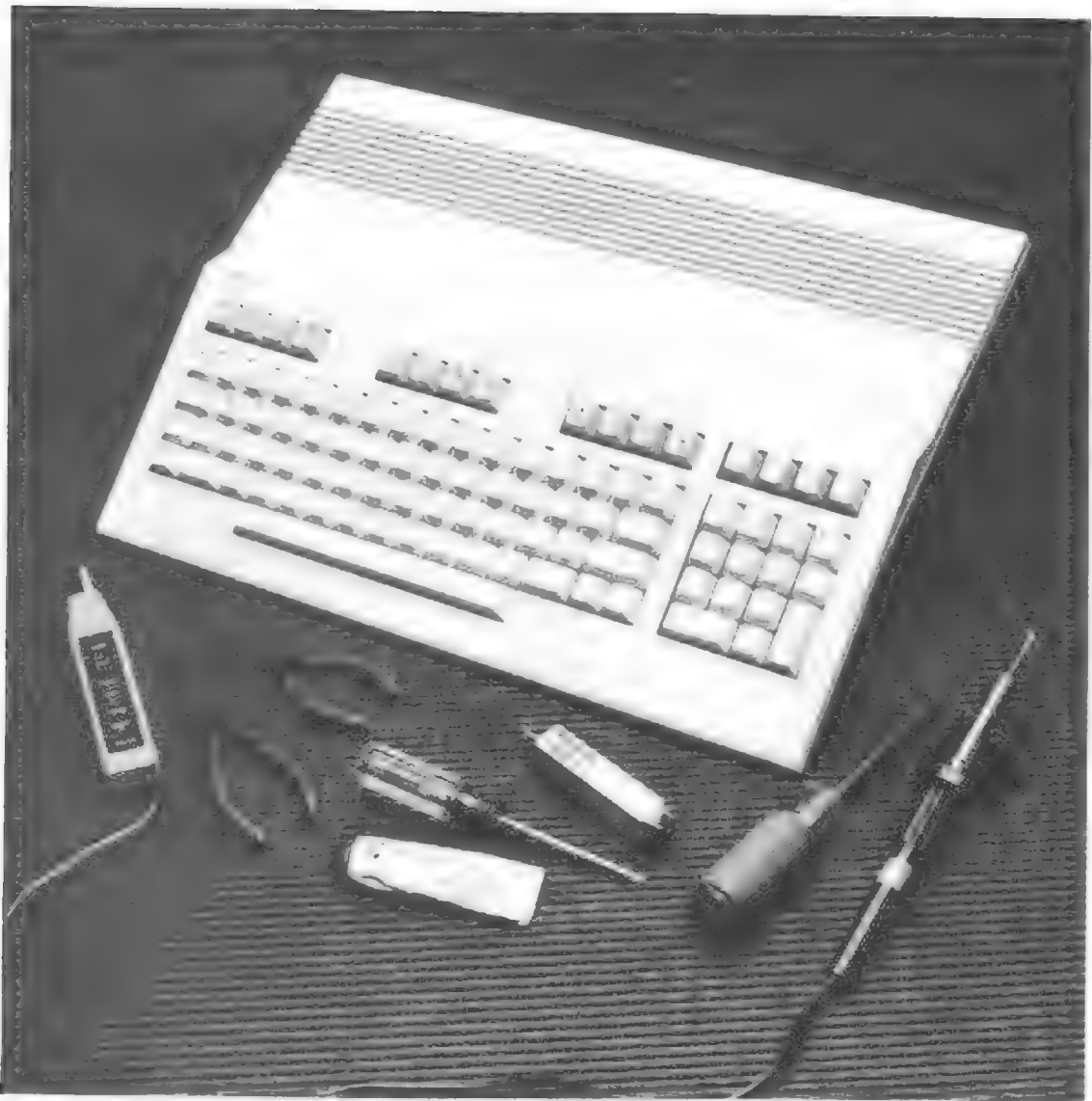
Fig. 2-1. To disassemble the C128, you need a number 10 Torx screwdriver, a Phillips head screwdriver, long nose pliers and a low-wattage soldering iron. For the reassembly, a tube of heat-transferring silicone paste should also be used. The logic probe, chip straightener-inserter and small cutters are also useful during troubleshooting.
